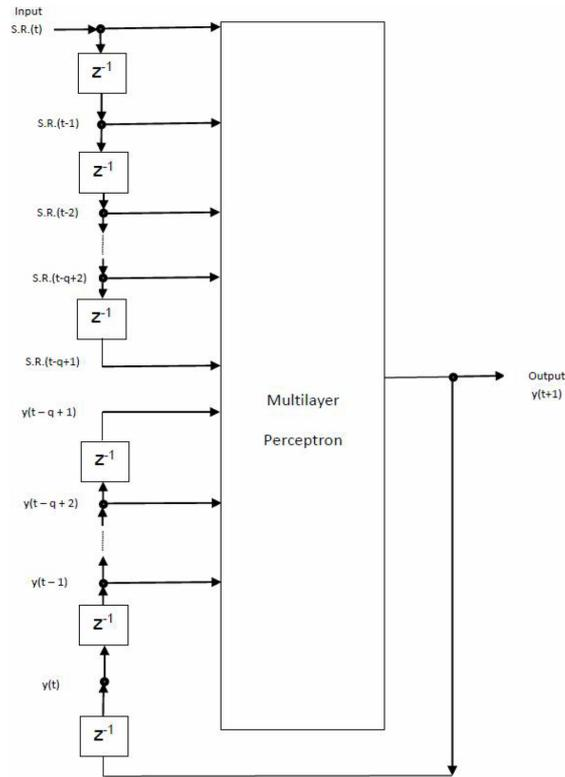
Figure 3: Architecture of the Non-linear Autoregressive Network (NARX) model [Cadenas et al., 2016].
