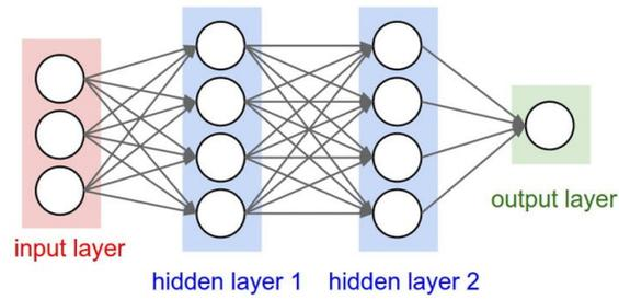
Figure 1: Artificial Neural Network - data are passed through a number of hidden layers before being output.
