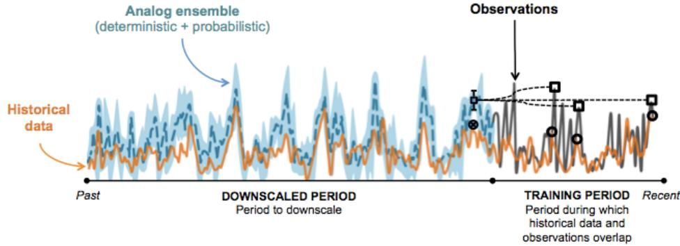
Figure 4: Analog ensemble method [NCAR, 2018]. Black dot - current value at time  $t$ . Black squares - observed values of the predictand for  $x$  best analogs.
